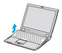
5 Lift the keyboard from the LCD display side, then gently turn it over on the touchpad space. Be careful not to detach the cable when lifting the keyboard.
